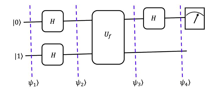
• The circuit that implements Deutsch's algorithm is shown above. We explain how it works in the following slides.
